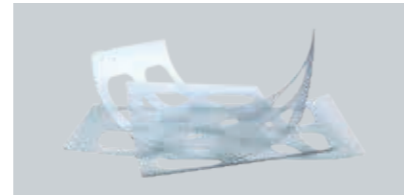
40% skeleton waste from thermoforming
