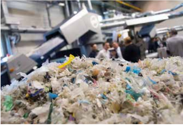
Washed and recycled PE film flakes: Raw material of the future for material producers © Erema
