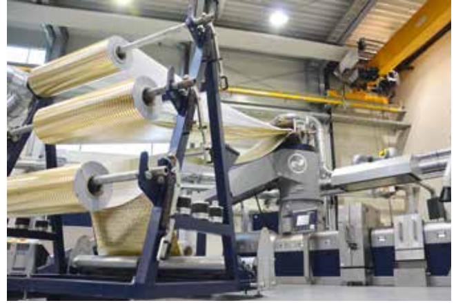
The Intarema TVEplus plant at the Erema Customer Centre adapts recyclates exactly to the respective customer wishes © Erema
