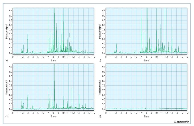
**Fig. 3.** Gas chromatography VOC analysis to assess odor optimization: The height and width of a peak are an indicator of the amount of the substance. a) Input material before extrusion process, b) after the preconditioning unit (before entering the extruder), c) after the extrusion process with Intarema TVEplus RegrindPro, d) after a further 7 h dwell time in the ReFresher (source: Fraunhofer IVV)
