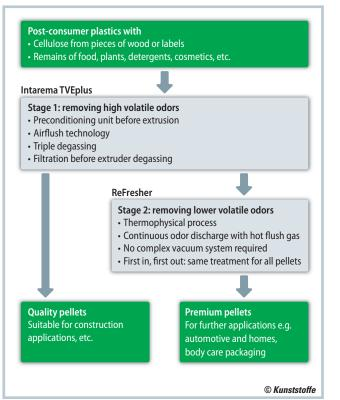
Fig. 1. Process overview: Odor-reduced pellets are created when not only the low molecular but also the low volatile, high molecular substances are removed (source: Erema)
