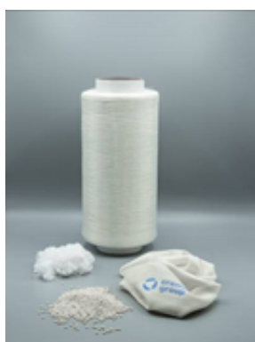
Photo: Fibre waste from filament fibre production was recycled into high-quality pellets in EREMA's fibre test centre. Using filament technology, a 3 dtex fibre was spun, which was processed into knitted fabric for clothing or technical textiles. (photo: EREMA)
