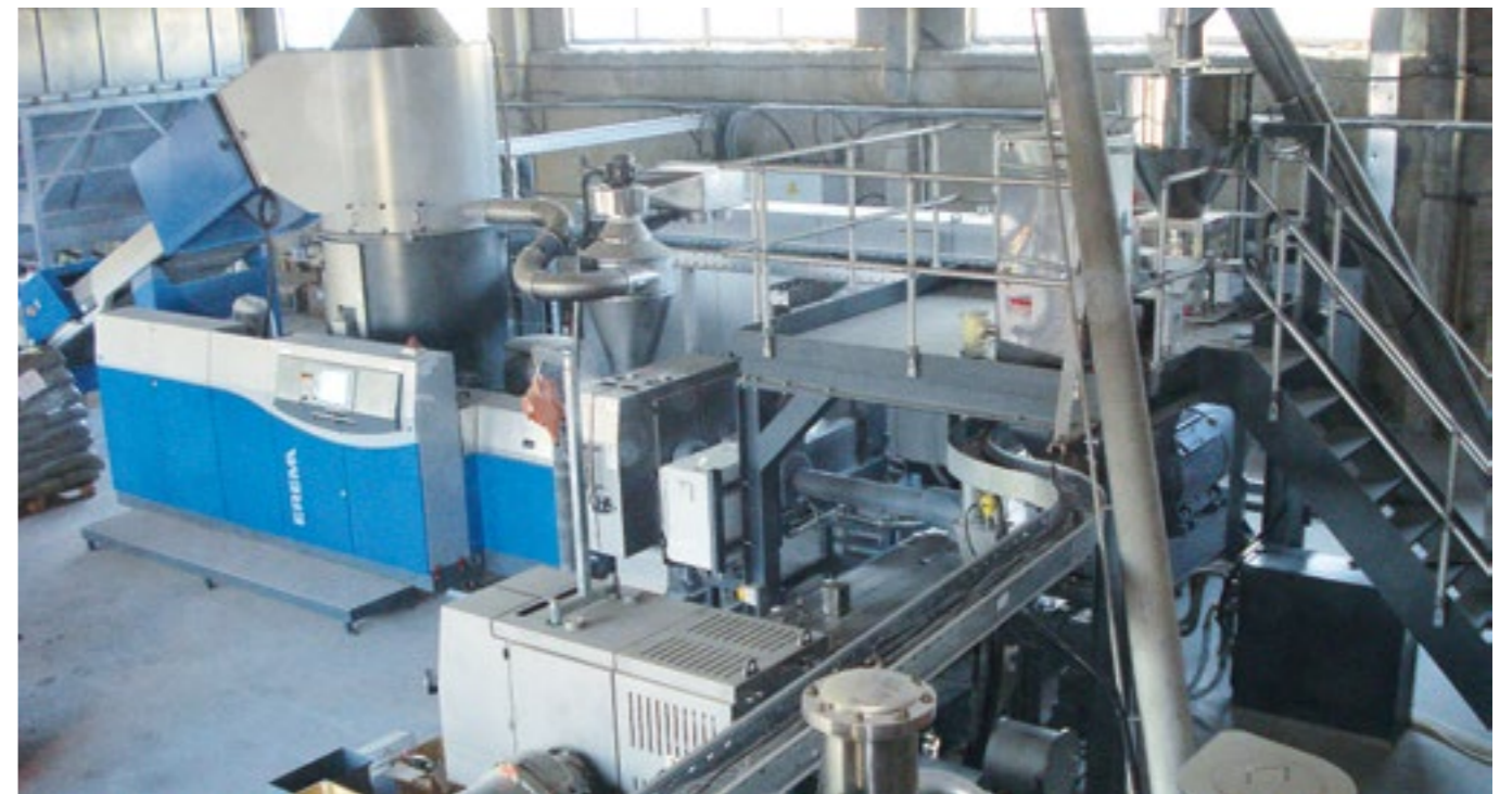
The combination of recycling and compounding with a COREMA® 1514 T enables the Russian company to produce exactly specified compounds from PP materials directly in a single pass. One particular benefit is the high degree of flexibility of the system with regard to different input materials.
