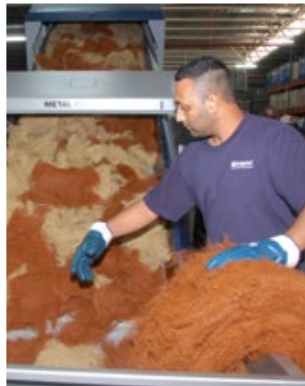
Belgotex uses the first INTAREMA® system to be employed in South Africa to recycle PP fibre and make high-quality pellets which are returned to the fibre production process.
