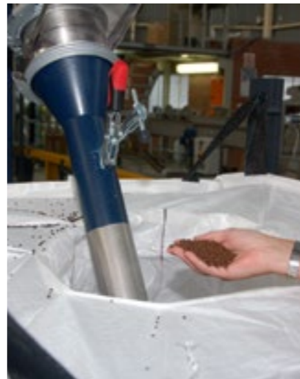
Belgotex uses the first INTAREMA® system to be employed in South Africa to recycle PP fibre and make high-quality pellets which are returned to the fibre production process.
