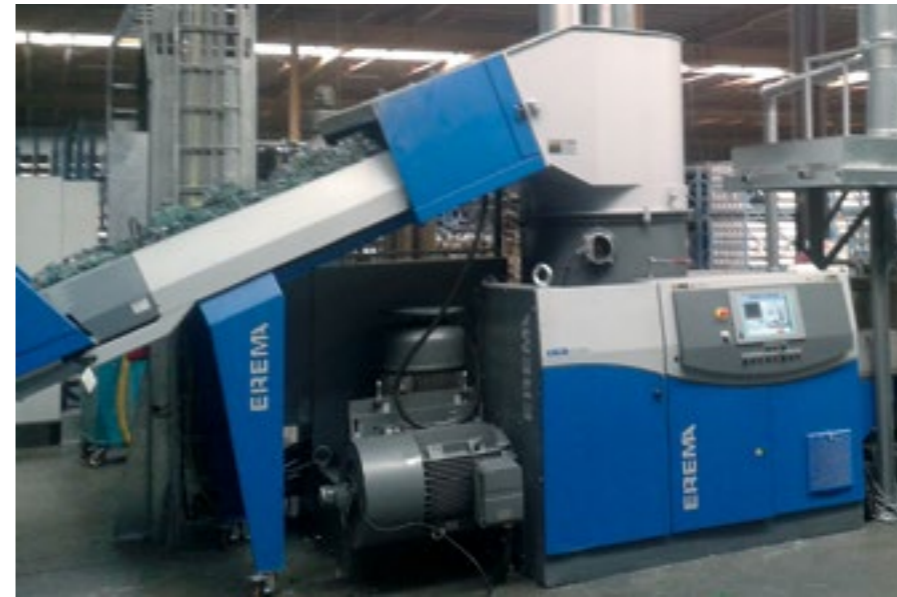
The COREMA® 1109 T system at Beaulieu Technical Textiles in Belgium enables efficient degassing of the spinning oil in the cutter/compactor.
