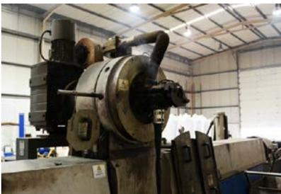
The EREMA Laserfilter in action: undesired impurities such as grass or straw are filtered out of the plastic melt continuously and reliably.
