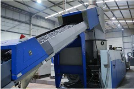
The EREMA 1514 TVE, which has been in operation since 2007, ensures high recycled pellet quality at Ambigroup Reciclagem in Chamusca, Portugal. The machine is equipped with Double Disc, Air Flush Module and Laserfilter.
