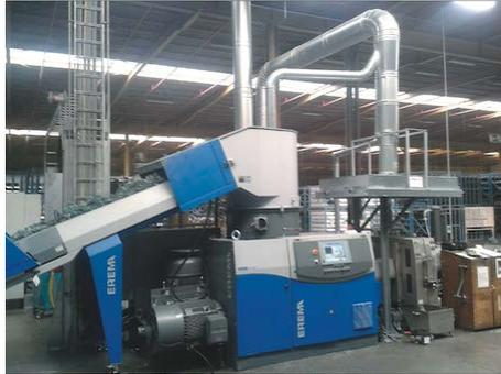
**The COREMA® 1109 T system at Beaulieu Technical Textiles in Belgium enables efficient degassing of the spinning oil in the cutter/compactor.**
