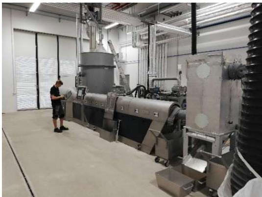
**Photo caption:** The recycling system is an application-specific combination of an INTAREMA 1512 TE recycling machine with a Lindauer DORNIER melt filter for fine filtration. Photo credit: DORNIER
