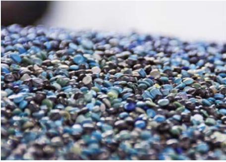
**100% recycled pellets from the company's own recycling lines are used for the production of bin liners**
