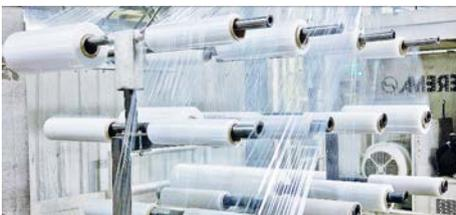
Each of the 70 extrusion machines at Polifilm is reconfigured several times a day, the scrap material is collected and sorted according to type and colour before it goes to a recycling machine
