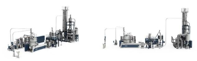
In the VACUNITE system, EREMA combines its VACUREMA® technology with the newly patented vacuum assisted nitrogen SSP from Polymetrix. Photo credit: EREMA
