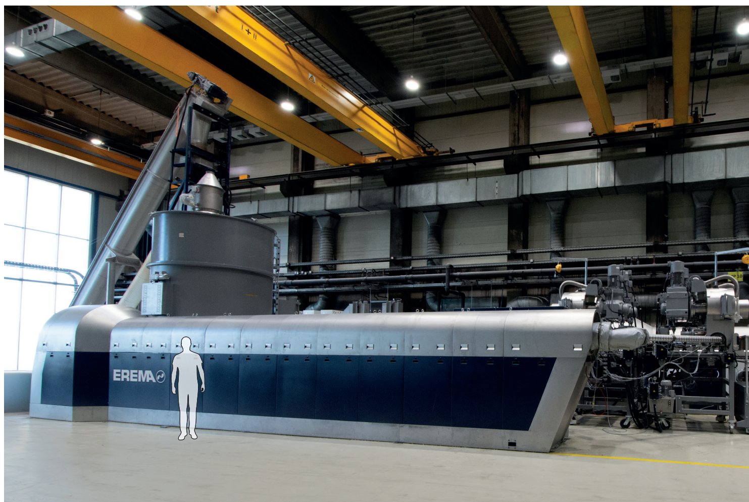
The INTAREMA® 2325 T-VEplus® RegrindPro® is the largest machine ever built for PO regrind and achieves a throughput of over 4 tonnes per hour.
