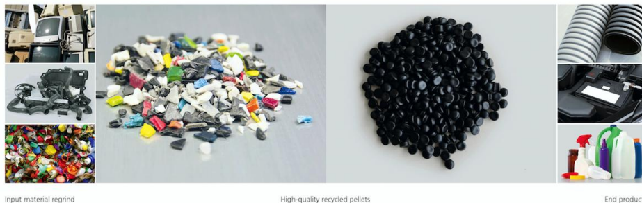
Fig. 2: Recycled pellets based on regrind material (thick-walled packaging, WEEE and automotive) represent an excellent alternative to virgin material for plastics processors.
