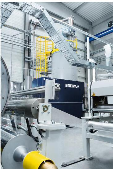
Fig. 2: Everything in a single working step: the input material goes from the MPR into the extrusion system and is then processed directly to make an inline sheet product.
