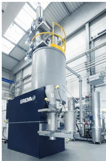
Fig. 3: The MPR from EREMA allows the decontamination, drying, dedusting and crystallisation of different PET input materials already prior to extrusion.
