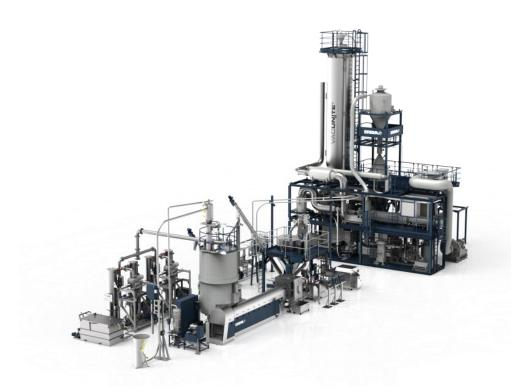
VACUNITE® systems see EREMA combine proven VACUREMA® technology with the vacuum-assisted nitrogen SSP from Polymetrix.
