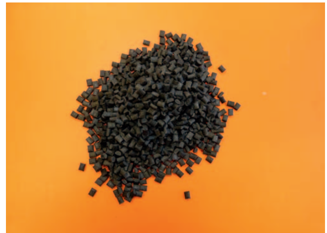
Fig. 8. PA6.6 recyclate with 30 % fibreglass and masterbatch black from PA6.6 fibres and airbag production waste
