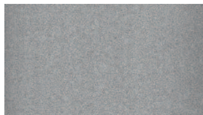
Fig. 4. Flat film sample (width 60 mm) produced on an OCS measuring extruder ME25/25D-V3; material: 23 % highly filled PP nonwoven/talc recyclate (talc content 70 % Omya Talco SD 20) + 77 % PP homopolymer
