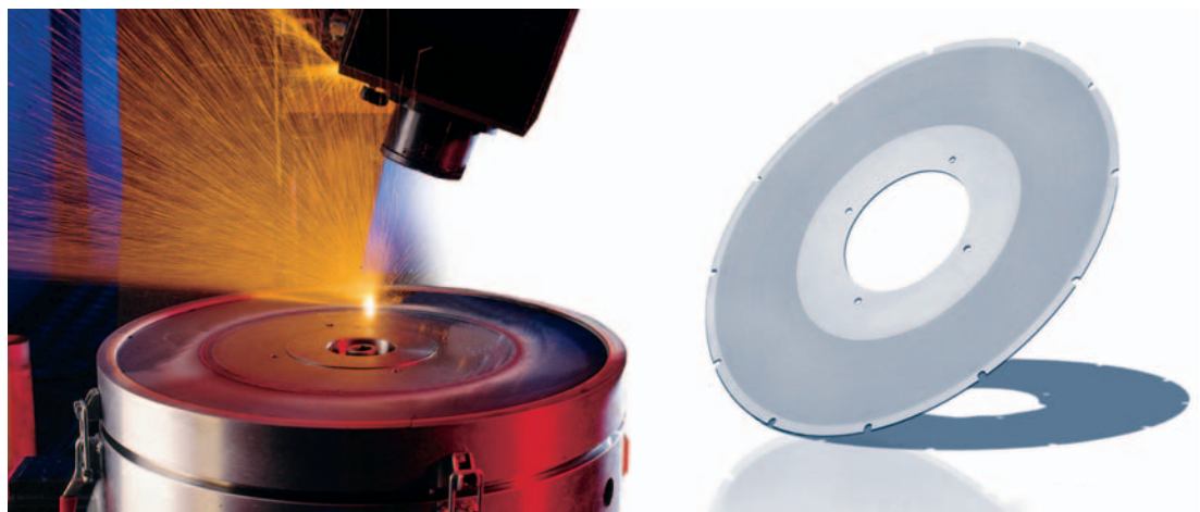
Fig. 5. Left: Conical holes are put into the filter screen using laser technology. Right: Hardened Laserfilter screen
