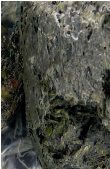
Fig. 6. The LF 4/350 achieves a thickening of 41 % in the filtration of washed PE shreds from the post-consumer collection system
