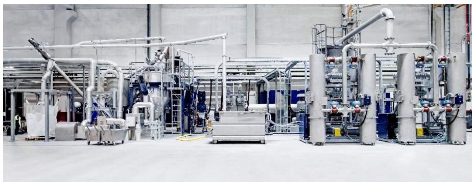
Photo: In the VACUNITE® system, EREMA combines its VACUREMA® technology with the newly patented vacuum assisted nitrogen SSP from Polymetrix. Photo shows the plant installed at RCS. Photo credit: EREMA
